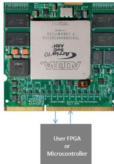
Fig. 8 SOC MPEG Codec Module connects to FPGA/microcontroller for user integration
