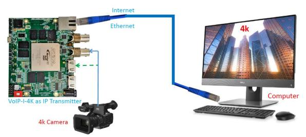
Fig. 5 Setup for evaluating the SOC encoder IP core using one VoIP-I-4K and a computer
