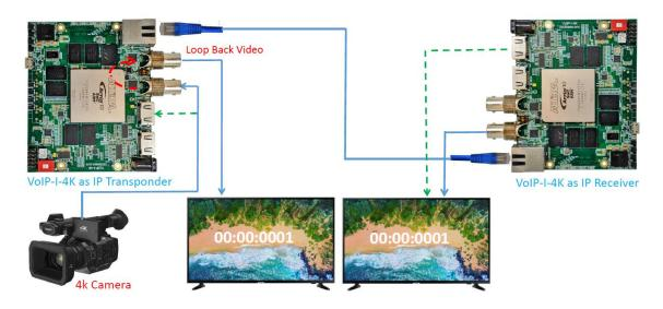
Fig. 7 Setup for testing the SOC encoder and decoder glass-to-glass latency
