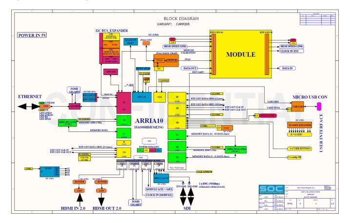
Fig. 8 Block diagram of VoIP-I-4K board
